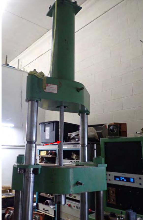
Figure 3-6: Photograph showing the load train utilized to test the intact service exposed conductor in uniaxial tension (the arrow indicates the conductor).
