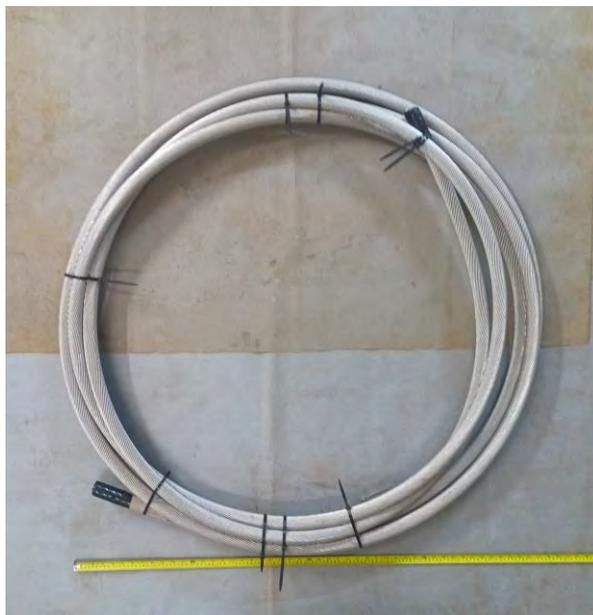
*Figure 3-1: Image showing the coiled length of the service exposed (used) conductor provided by NL Hydro as received for analysis.*
