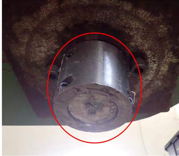
Figure 3-5: Photograph showing the epoxy filled socket fixture (ellipse) utilized to terminate the conductor at both ends.
